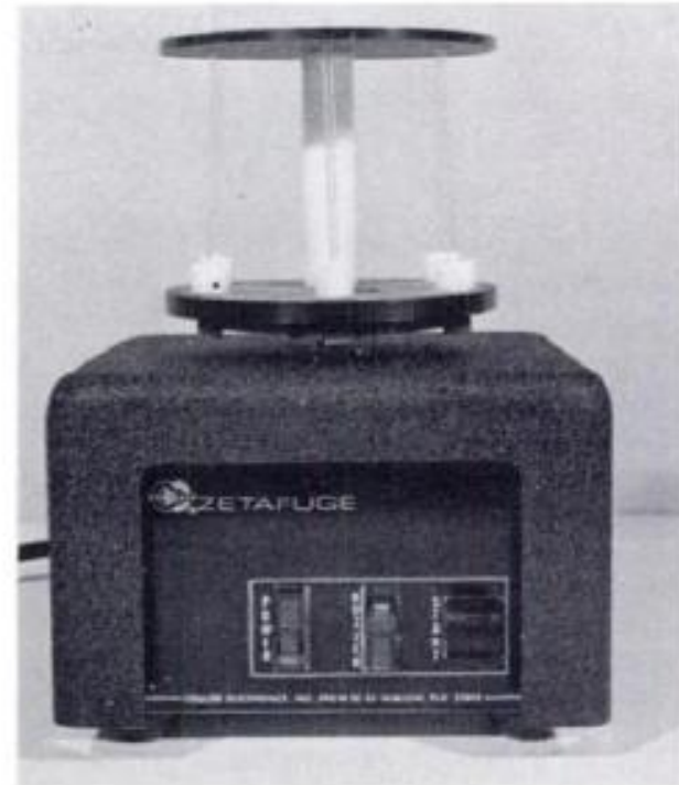
Fig. 2. Photograph of Zetafuge, the centrifugal device that produces the repetitive cycles of compaction and dispersion.
